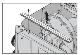
Figure 26. Remove Gasket Retainer Bracket
