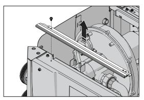
Figure 5. Remove Gasket Retainer Bracket
