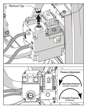
Figure 33. Adjust Offset Pressure
