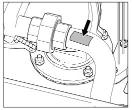
Figure 11. Affix Converted Fuel Type Sticker onto the Gas Train
