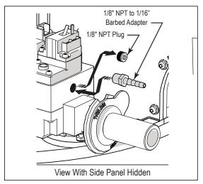
Figure 16. Remove NPT Plug and Insert Barbed Adapter
