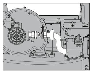
Figure 9. Remove the Gas Orifice
