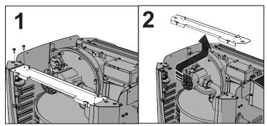
Figure 7. Remove Rear Brace Bar
