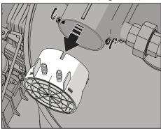
Figure 12. Remove Air Intake Orifice
