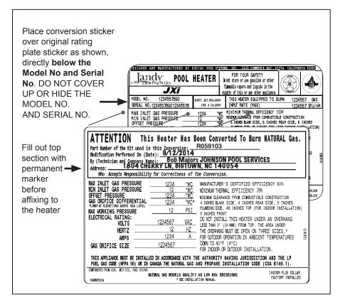
Figure 22. Correct Placement of the Converted Fuel Type Data Rating Plate Sticker
