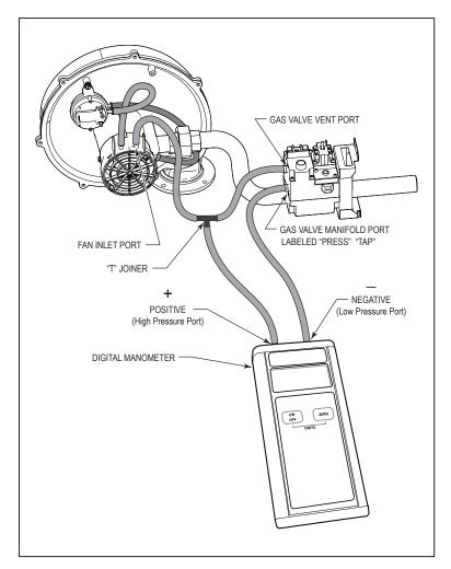
Figure 20. Testing Gas Offset Pressure
