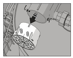
Figure 39. Replace the Air Intake Orifice
