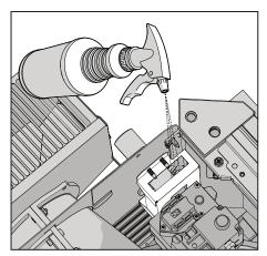
Figure 15. Spray Soap Solution for Leak Test
