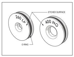
Figure 31. Etched Surface of Gas Orifice
