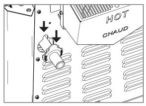
Figure 19. Line Up Tab with Gas Pressure Tap Port
