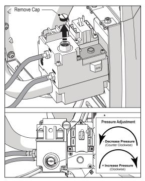
Figure 21. Adjust Differential Offset Pressure
