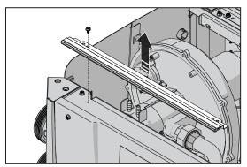
Figure 36. Remove Gasket Retainer Bracket
