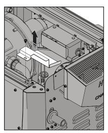
Figure 35. Remove Gas Valve Bracket
