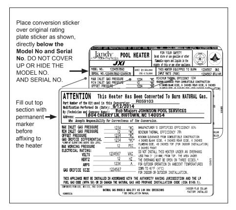
Figure 2. Correct Placement of the Converted Fuel Type Data Rating Plate Sticker
