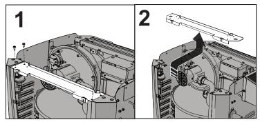
Figure 28. Remove Rear Brace Bar
