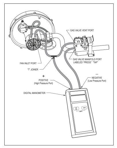
Figure 32. Testing Gas Offset Pressure
