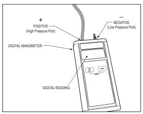
Figure 18. Test the Gas Inlet Pressure
