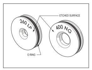
Figure 10. Etched Surface of Gas Orifice
