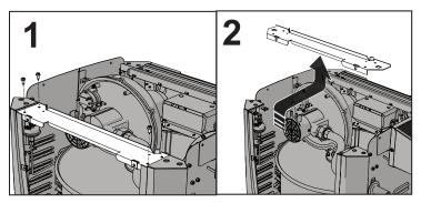
Figure 38. Remove Rear Brace Bar
