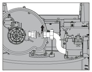
Figure 30. Remove the Gas Orifice
