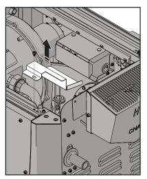
Figure 4. Remove Gas Valve Bracket
