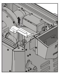
Figure 25. Remove Gas Valve Bracket
