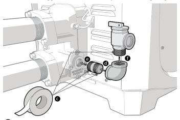
**(**) Install the pressure relief valve. Make sure to get a sung fit. Do not overtighten.
