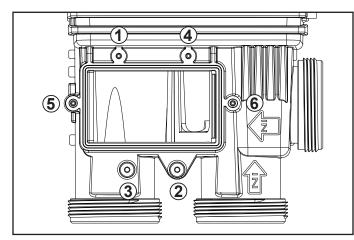
Figure 24. Header Bypass Reassembly Torque Pattern
