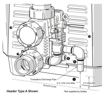
**NOTE:** Hardware showing in dotted line is not provided by Zodiac. Pressure Relief Valve hardware is provided on ASME heater models only.
