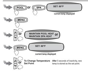
If connected, the Maintain Heat mode monitors the pool water temperature 24 hours a day by turning the pool pump on and sampling the water temperature. When the water temperature drops below the programmed temperature set point, the controller automatically starts heating the pool.
