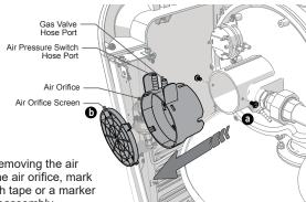
**TIP:** When removing the air hoses form the air orifice, mark the hoses with tape or a marker to help with reassembly.
