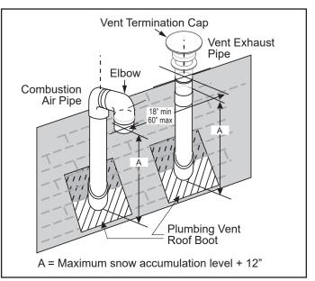
Figure 6. Vent and combustion air terminals at roof.
