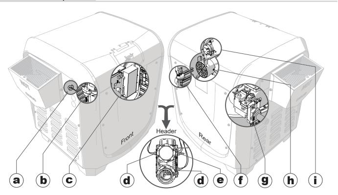
(a) Flue Temperature Sensor Monitors temperature at the exhaust flue. If excessive temperatures are detected, combustion will stop and a fault will be displayed.
