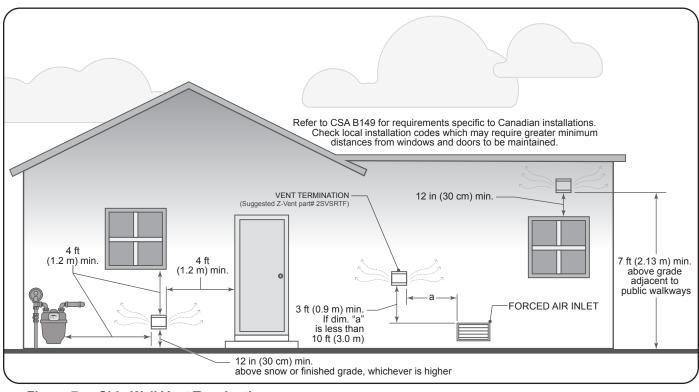
Figure 7. Side Wall Vent Termination
