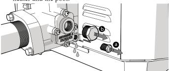
**a** Remove drain plug from header and allow all water to drain from heat exchanger.
