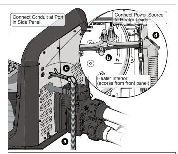
**NOTE:** If the heater is converted to accept 120V, the "Hot" wire of the 120V power supply has to be connected to the black wire (ACH1) on the power distribution board and the "Neutral" wire of the 120V power supply has to be connected to the red wire (ACN1) of the power distribution board. Please see *Figure 15* for details.
