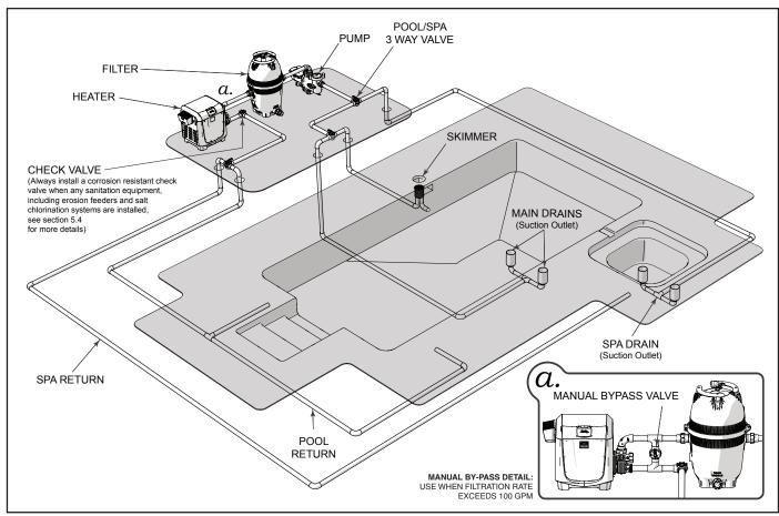
Figure 9. Typical Water Piping Configuration
