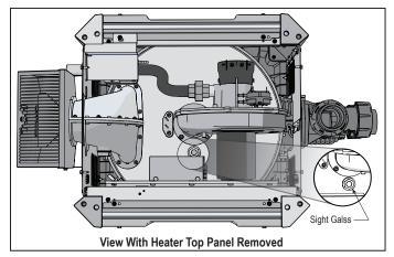
Figure 23. Remove Heater Top to View Sight Glass
