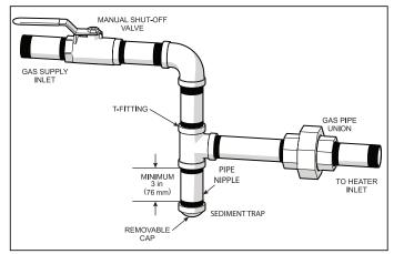
Figure 8. Manual Shut-off Valve and Sediment Trap
