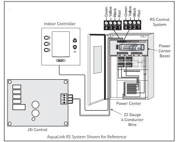
Figure 16. Wiring the JXi to a Zodiac<sup>®</sup> Remote
