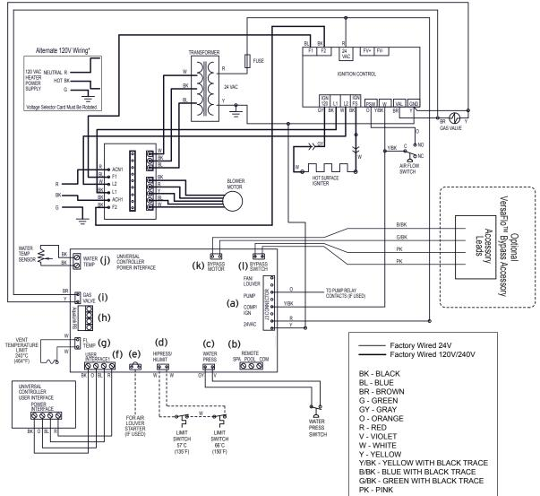
Figure 15. JXi Connections/ Schematic Wiring Diagram
