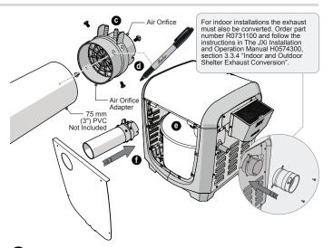
C Align the orifice adapter with the orifice tabs and secure with four screws.
