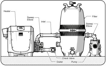
Figure 11. Versa Plumb Heater Inlet
