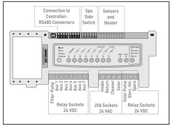
Figure 18. AquaLink RS PCB with firmware REV N or higher
